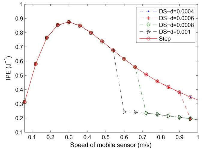
Fig. 10. IPE of delayed step utility approaches that of step utility as  $d$  becomes small.
