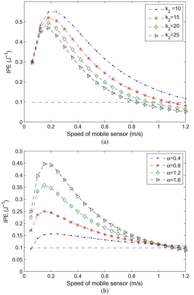
Fig. 5. Impact of energy model on the IPE for events that have exponential utility function. (a) IPE as a function of  $v$  for different  $k_2$ 's. (b) IPE as a function of  $v$  for different  $\alpha$ 's.
