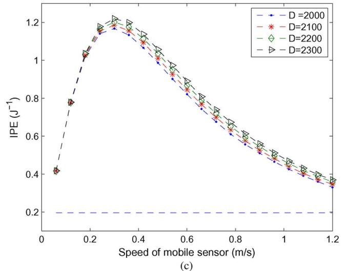
Fig. 3. Impact of PoI distribution on the IPE for the step utility function. (a) IPE as a function of  $v$  for different  $n$ 's. (b) IPE as a function of  $v$  for different  $D$ 's. (c) IPE as a function of  $v$  for different  $D$ 's while fixing  $\gamma$ .
