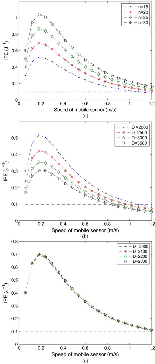
Fig. 6. Impact of PoI distribution on IPE for the exponential utility function. (a) IPE as a function of  $v$  for different  $n$ 's. (b) IPE as a function of  $v$  for different  $D$ 's. (c) IPE as a function of  $v$  for different  $D$ 's while fixing  $\gamma$ .
