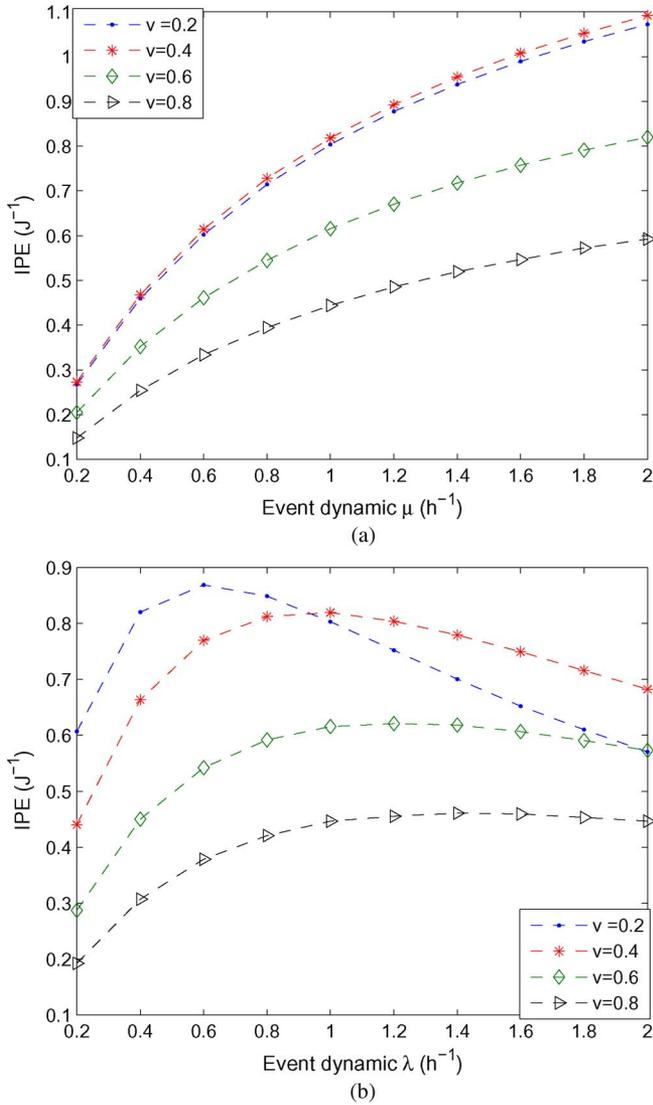
Fig. 4. Impact of event dynamics on the IPE for the step utility function. (a) IPE as a function of  $\mu$  for different  $v$ 's. (b) IPE as a function of  $\lambda$  for different  $v$ 's.
