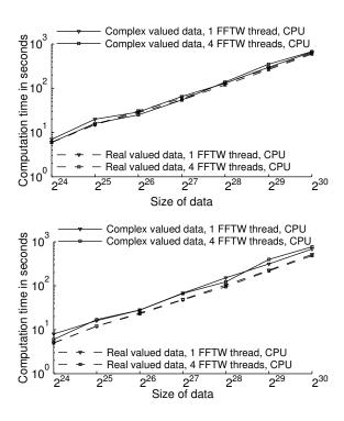
Figure 7: Runtimes for the forward (top) and inverse (bottom) 5D wave atom transform as the function of data volume.
