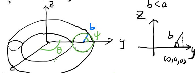
$$T_\psi = \left\langle (-b\sin\psi)\cos\theta, (-b\sin\psi)\sin\theta, b\cos\psi \right\rangle$$
